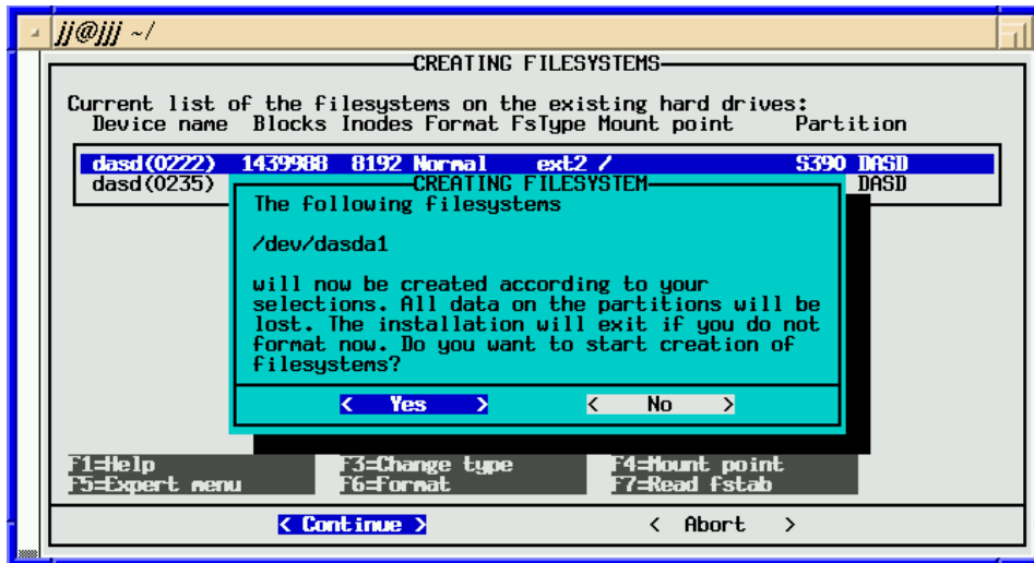
Figure 54. YaST: confirmation before actually creating file systems
