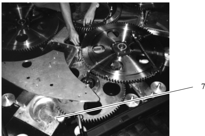
Fig. 9-49: Play of the Tooth Profile on the Main Tower
