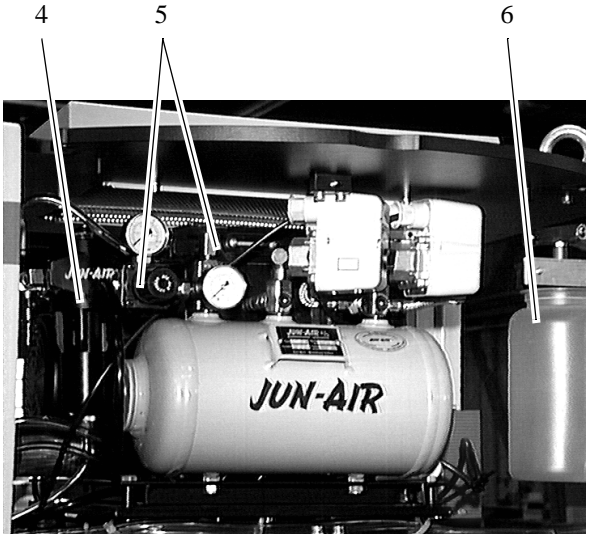
Fig. 8-22: Compressed Air Supply
