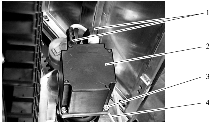
Fig. 9-47: Auxiliary Tower Drive-Motor
