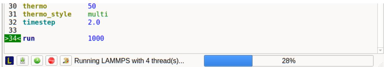
While LAMMPS is running, the contents of the status bar change. On the left side there is a text indicating that LAMMPS is running, which also indicates the number of active threads, when thread-parallel acceleration was selected in the *Preferences* dialog. On the right side, a progress bar is shown that displays the estimated progress for the current *run* or *minimize* command.
