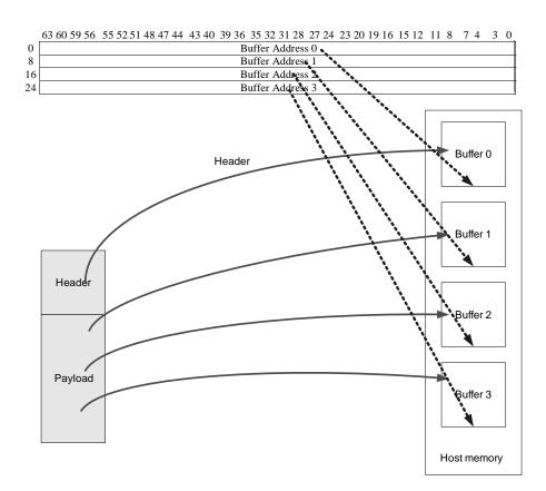
Figure 3-2. Header Splitting
