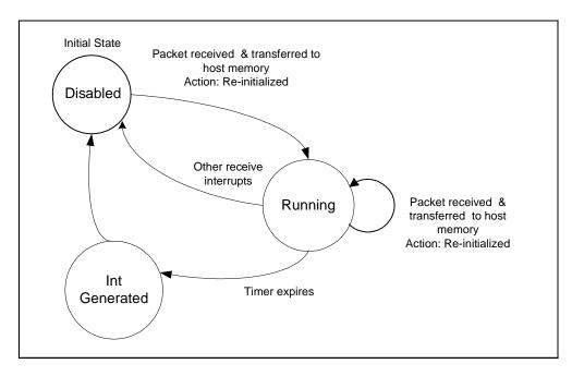
Figure 3-4. Packet Delay Timer Operation (State Diagram)
