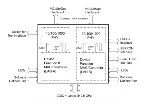
Figure 2-1. 82571EB/82572EI External Interface
