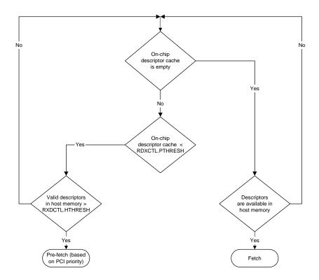
Figure 3-3. Receive Descriptor Fetching Algorithm
