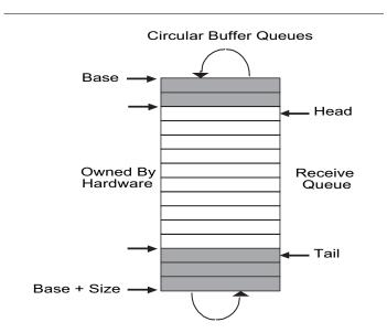
Figure 3-1. Receive Descriptor Ring Structure
