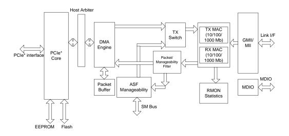
Figure 2-4. Internal Architecture Block Diagram
