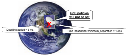
Figure 3: Inconsistent QoS Policies for an MMS Ground Station
